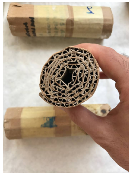
Fig. 1. The cardboard traps (15×40 cm) used to collect the PRM.
